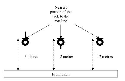
B.3.2 Position of the jack alongside a 2-metre measuring device
